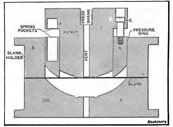
Fig. 5. Triple-action Die for Drawing Spherical-shaped Covers
